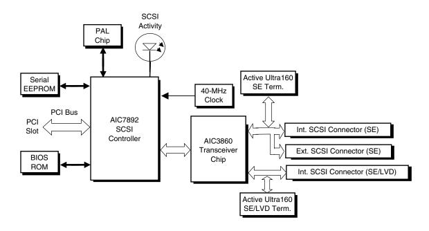
Figure G–2. Compaq/Adaptec Ultra SCSI Adapter Card Block Diagram
